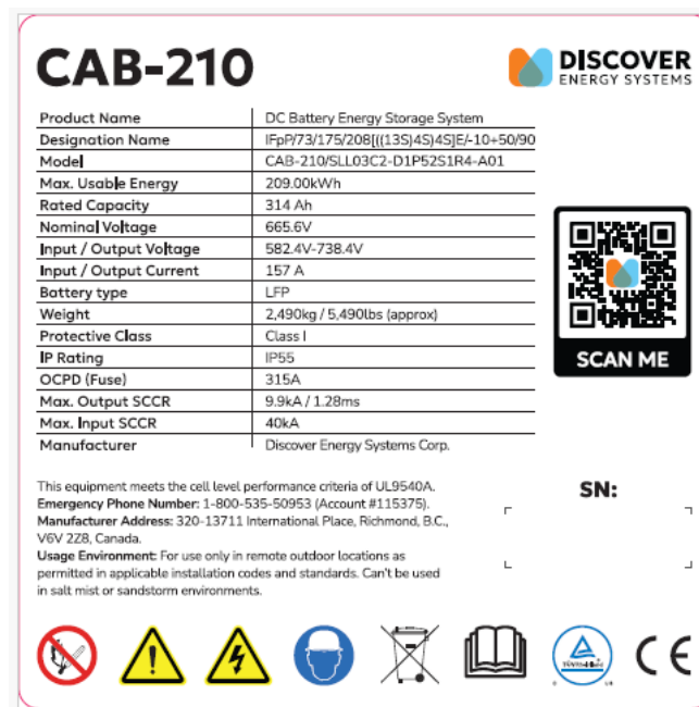
Outdoor Cabinet Nameplate
